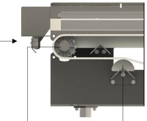
Solid round idler / drive shaft Keyed precision machined solid round shaft for added strength and longevity.
