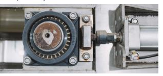
Self-adjusting pneumatic take-up for maintenance-free belt tensioning. Horizontal mounting offers improved response to changing demands with double take-up length and lower profile design.
