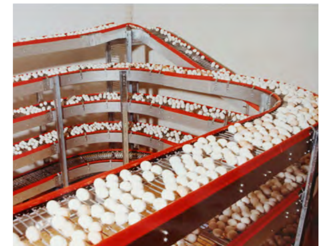
With the curve conveyor completely new and flexible barn layouts could suddenly be realized.
